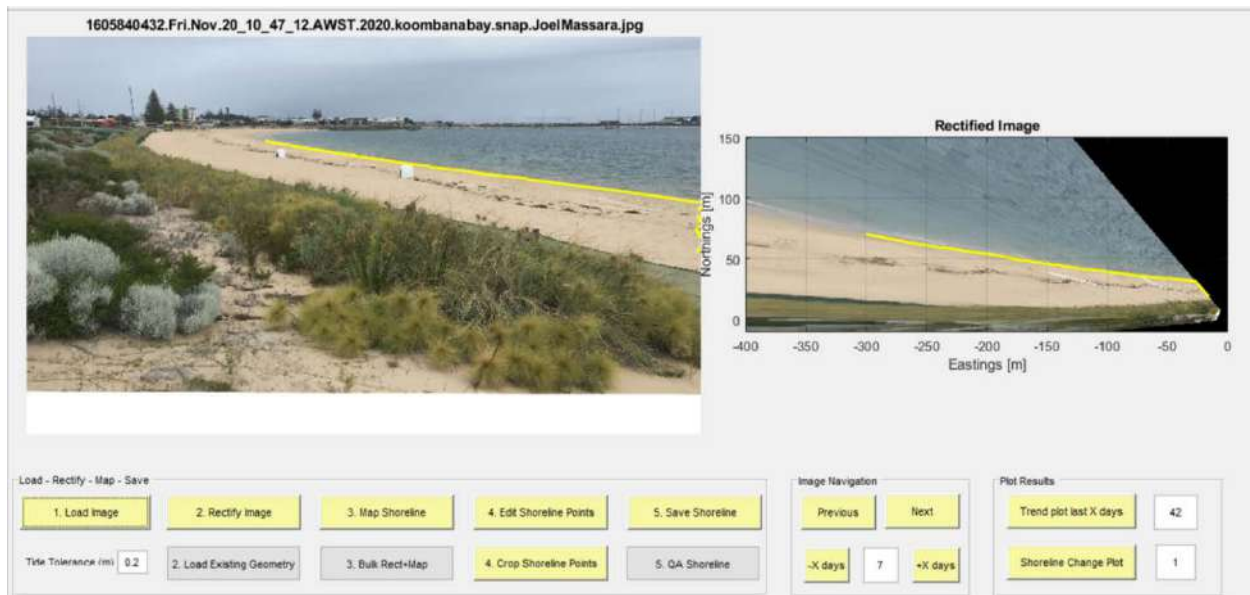
Figure 4. Example CoastSnapWA workflow using the Graphical User Interface (GUI). Example is from Koombana Bay from 20 November 2020. User image is displayed on the left, rectified image on the right and mapped shoreline displayed in yellow on both images.
